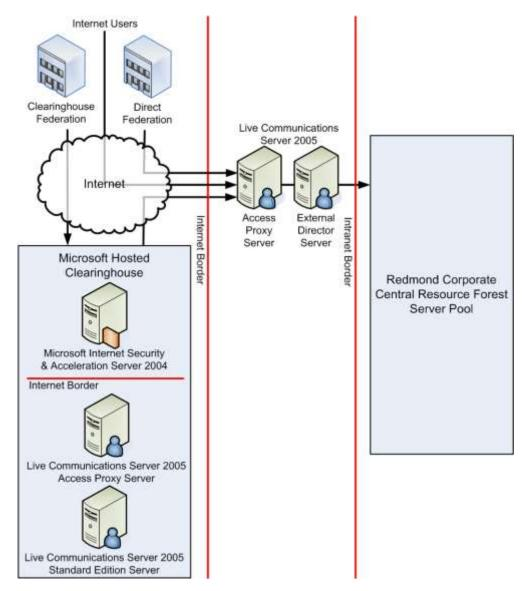
Figure 5. Remote user and federated access physical architecture
