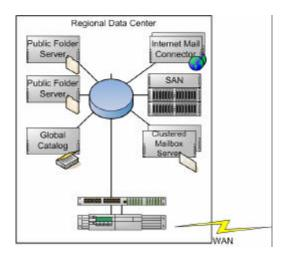
Figure 5. Typical post-consolidation configuration
