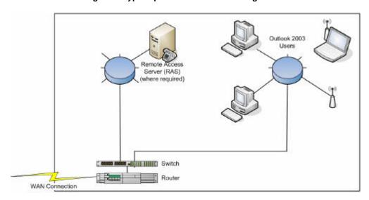
Figure 6. Typical post-consolidation local office configuration
